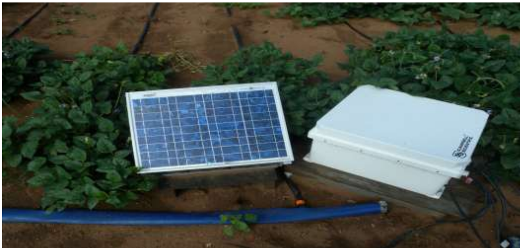
Plate 4: A TDR regularly used for in-situ soil moisture monitoring on the field
