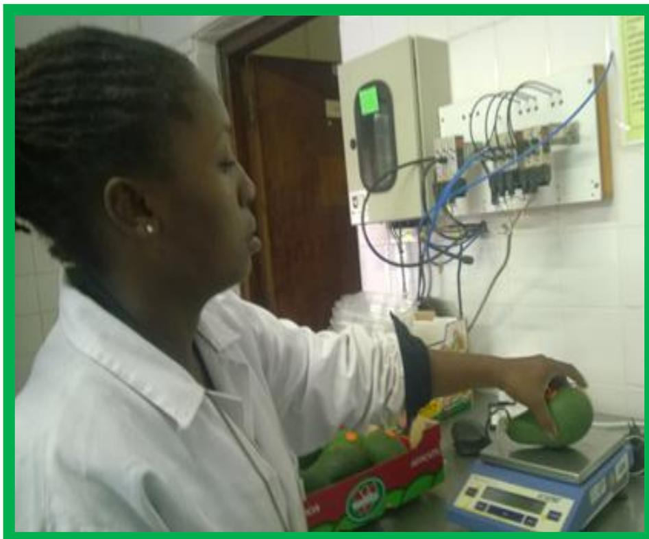
Figure 3.3 Weighing new 'Fuerte-type' avocado fruit for mass loss
