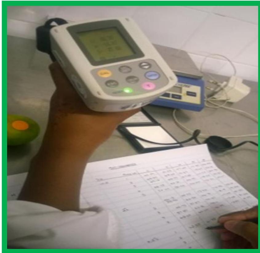
Figure 3.4 Measuring the colour parameters of the new 'Fuerte-type' avocado fruit
