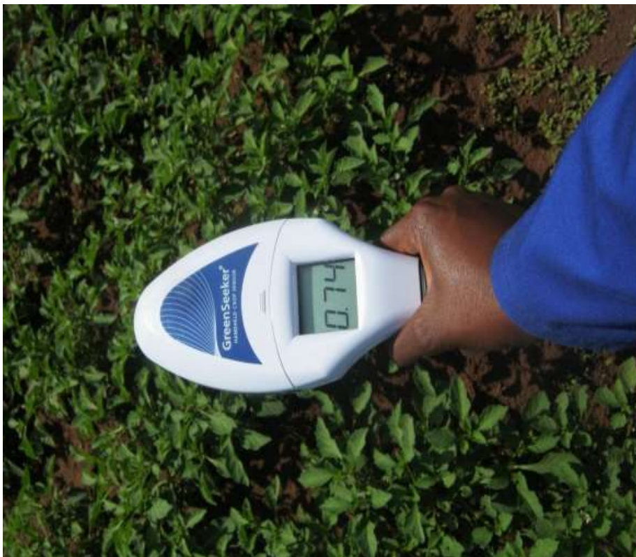
Figure 4.4: Measuring plant vigour using a hand-held green seeker
