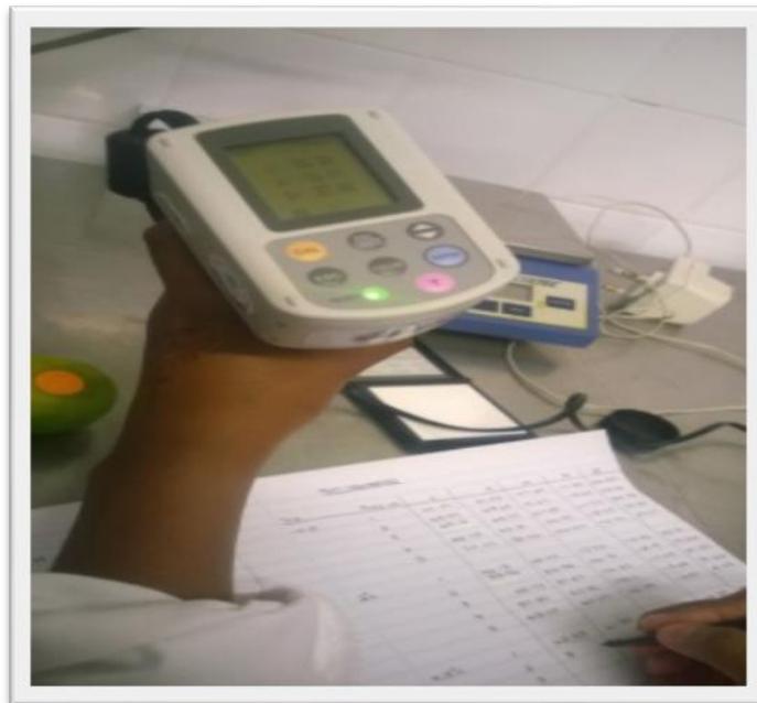
Figure 3.2 Chromameter used to measure 'Hass' avocado fruit skin colour parameters (lightness ( L^* ), a^* and b^* values)
