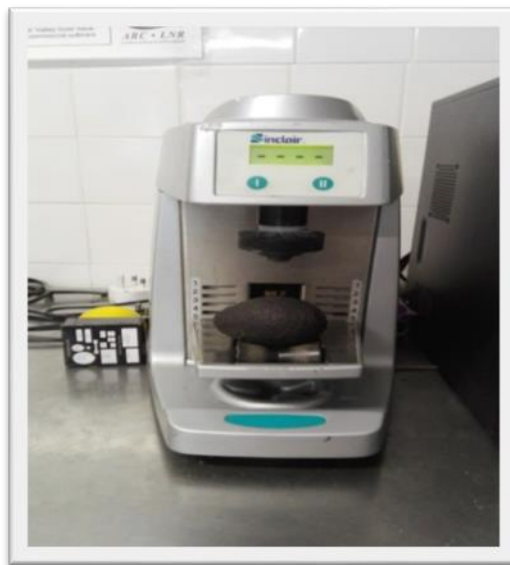
Figure 3.3 Sinclair IQ™ automated desktop firmness machine used to measure firmness of 'Hass' avocado fruit
