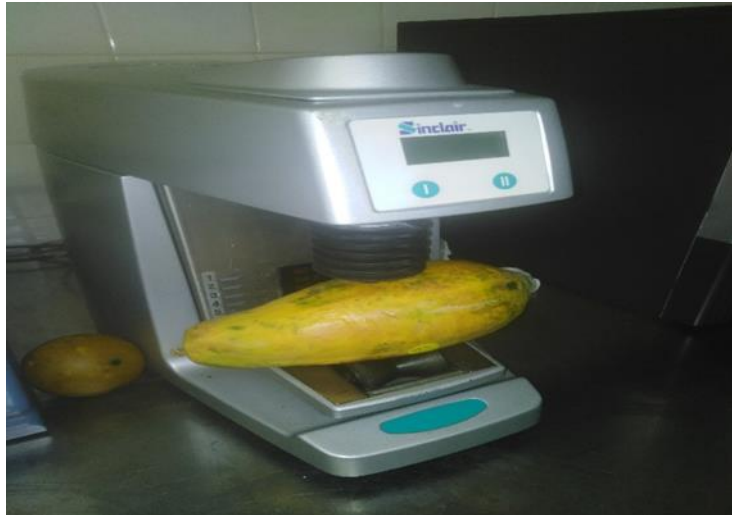
Figure 3.2: Sinclair IQ™ automated desktop machine used to measure 'Solo' papaya fruit firmness
