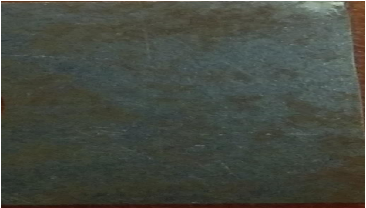
Figure 4. 11: Mild steel before corrosion testing.
