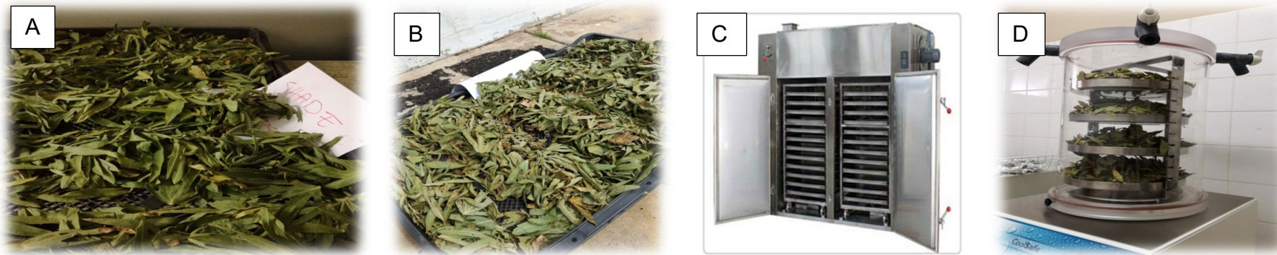
Figure 3.2: Jatropha zeyheri drying methods, A) Shade-drying, B) Sun-drying, C) Oven-drying and D) Freeze-drying
