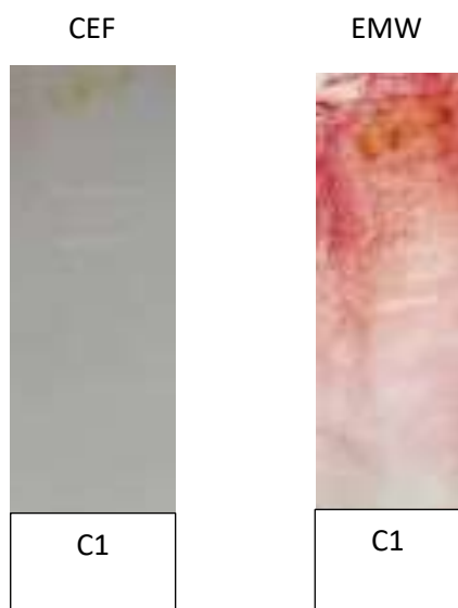
Figure-8.3-Bioautograms-of-10-isopropyl-4,4-dimethylhexadecahydro-1H-cyclopenta [b]phenanthren-3-ol developed in CEF (left) and EMW (right), sprayed with C. albicans . White areas indicate inhibition of fungal growth.
