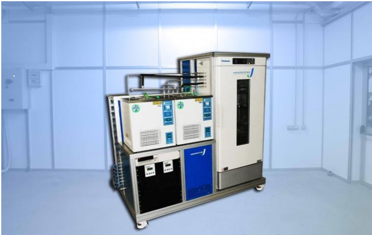
Figure 3.12: Schematic diagram of an installed KENOSISTEC KSGAS6S gas sensor station [39].
