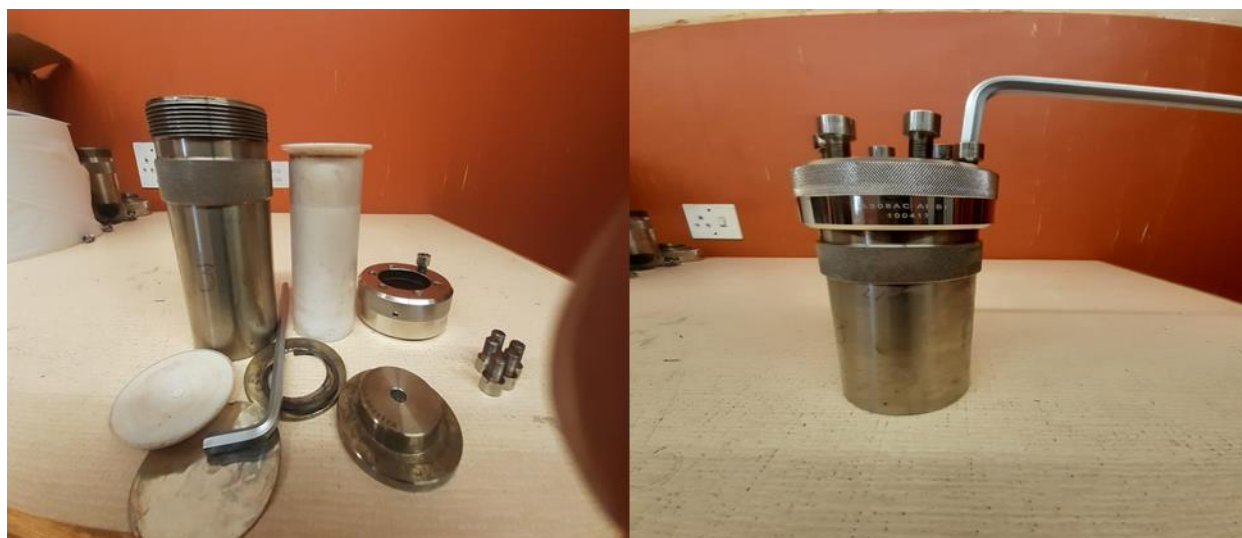
Fig. 3.9. Stainless steel autoclave with the inner part Teflon liner.
