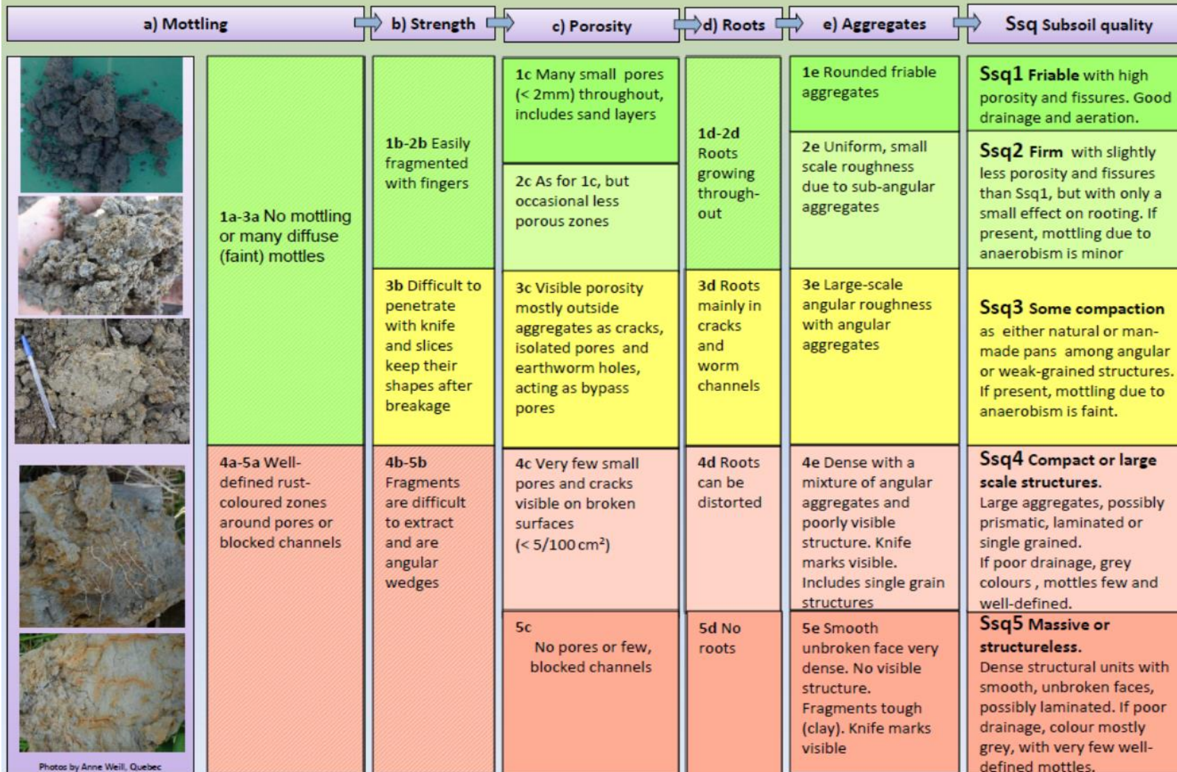
Figure 3.2a. Subsoil Visual Evaluation of Soil Structure (SubVESS) flowchart (Ball et al., 2015).
