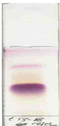
Figure 3.10b: TLC chromatogram to check the purity profile of the fraction obtained from pooled tubes (13-18) with similar chromatographic properties.
