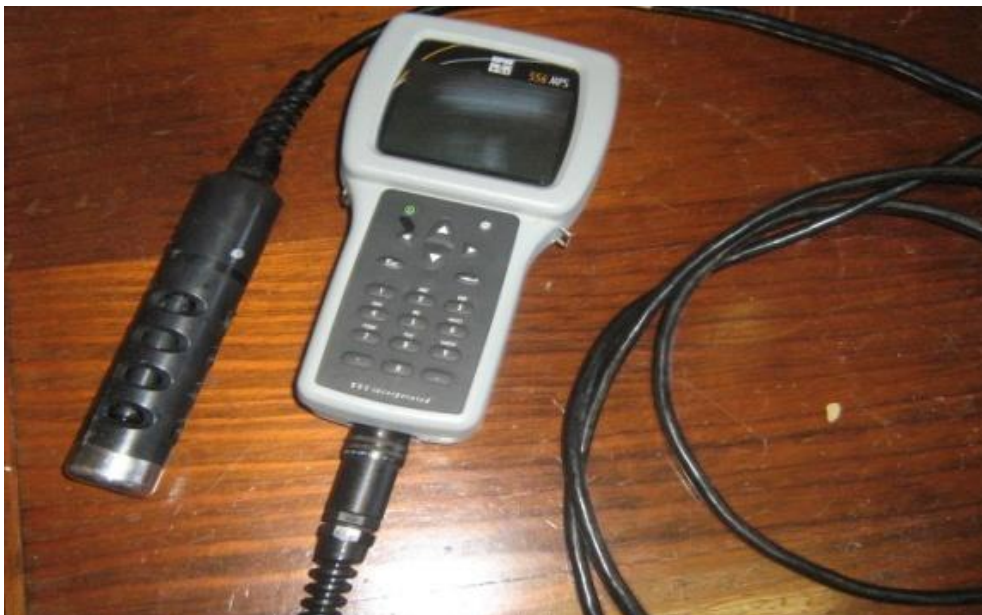
Figure 3.4: Hand held YSI meter used for measuring water quality parameters.
