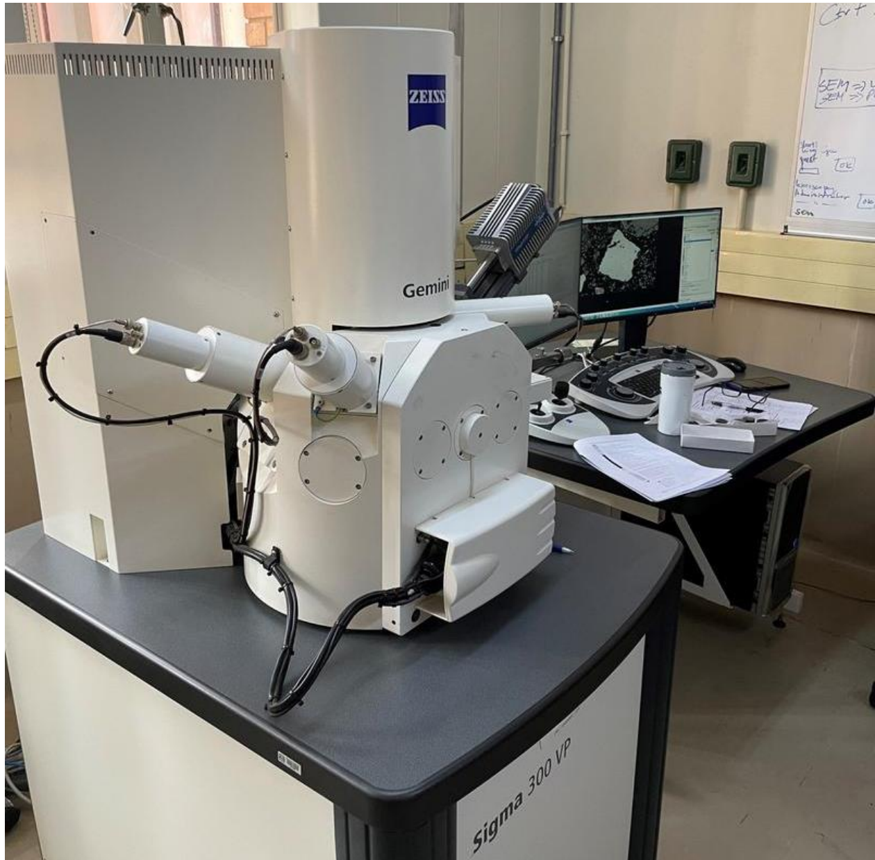
Figure 3.4: Scanning Electron Microscopy fitted with Energy Dispersive X-ray Spectroscopy.
