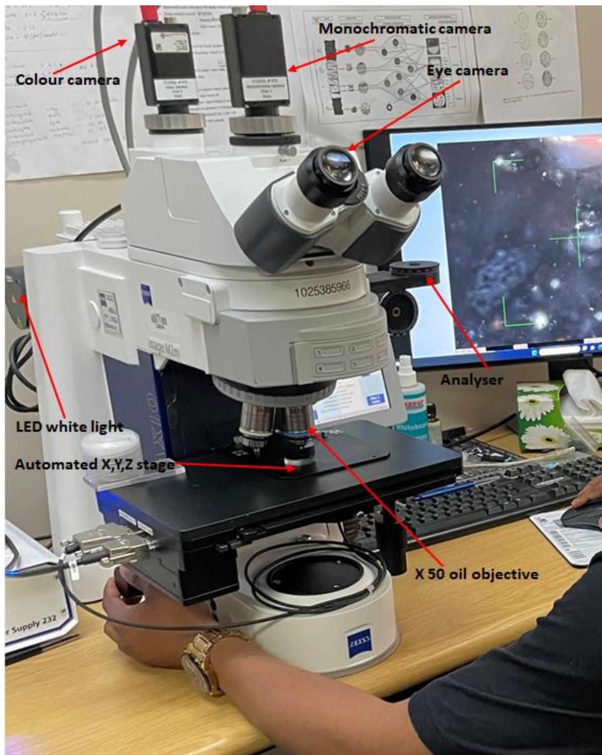
Figure 3.2: Photograph showing a zeiss Axio Imager M2 polarised reflected light microscope equipped with Hilgers diskus Fossil software.
