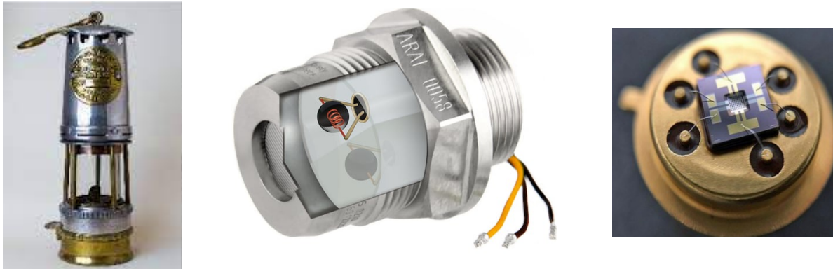
Fig. 1.1: Images showing (a) flame safety light, (b) catalytic sensor and (c) chemiresistive sensor [1.1.-1.3].
