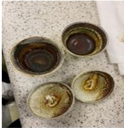
Figure 2.8 Photo of melted \text{Na}_2\text{SO}_4 when heated to 1000 °C (Mashigwana, et al. , 2022).
