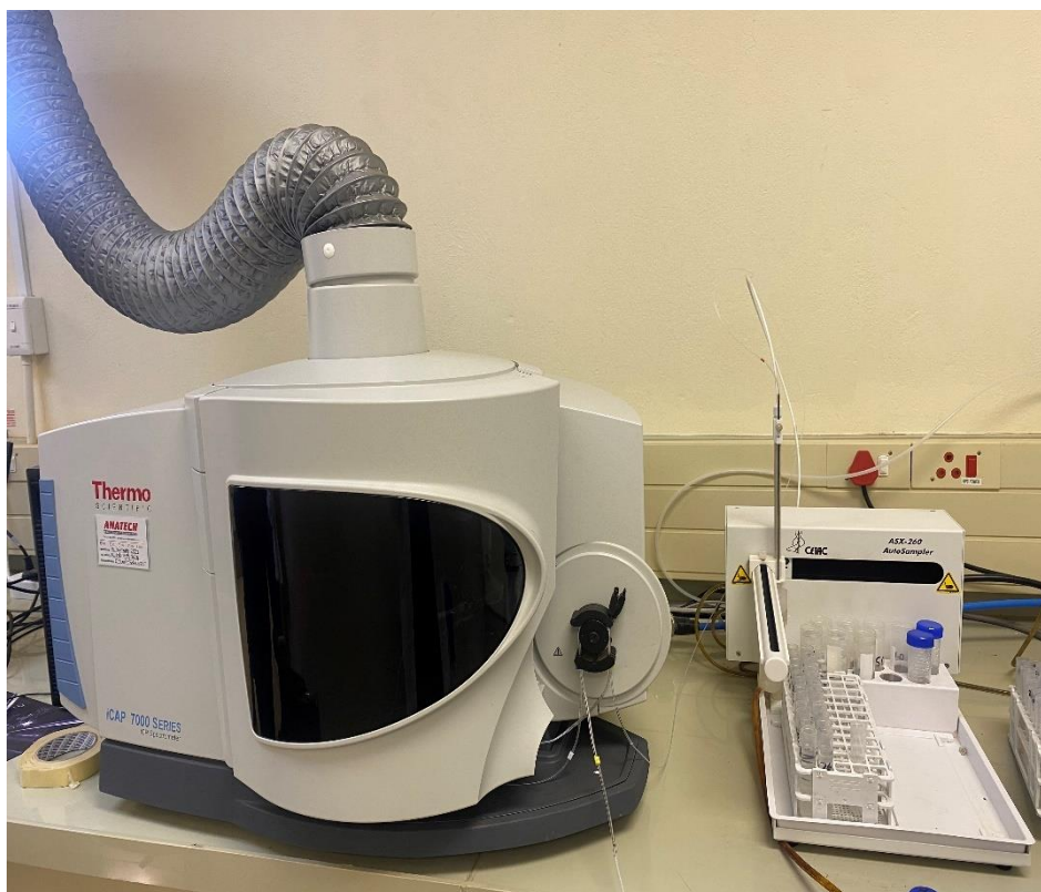
Figure 3.7 Inductively coupled plasma optical emission spectrometry (Courtesy of C P Mokgohloa)
