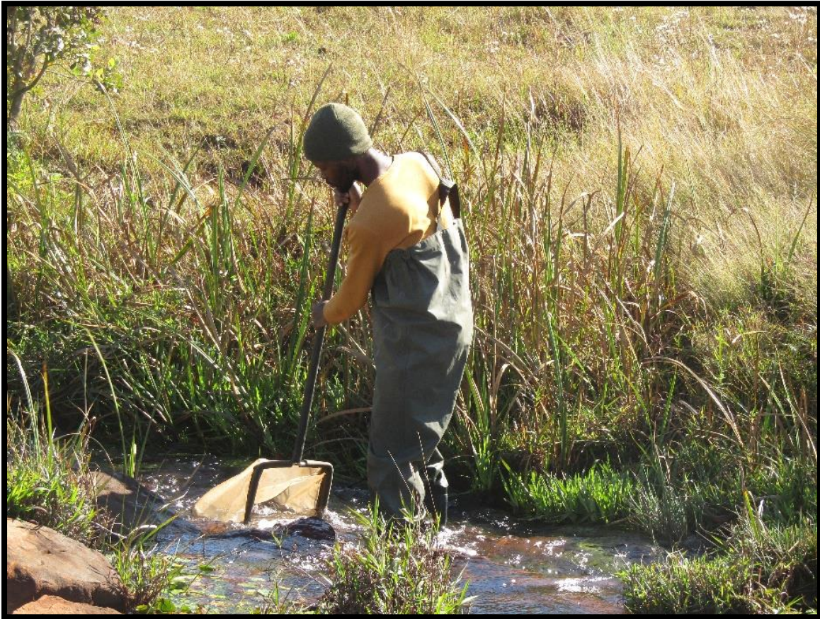
Figure 2.16: Collecting macroinvertebrates using a SASS net.
