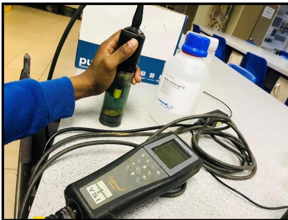
Figure 2.13: YSI meter used to measure physico-chemical parameters.
