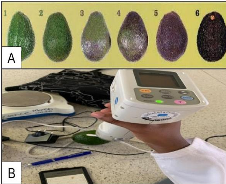
Figure 3.2 Measurements of colour using subjective and objective measurements (A= Visual colour rating, B= colour measurement using chromameter) in ‘Hass avocado
