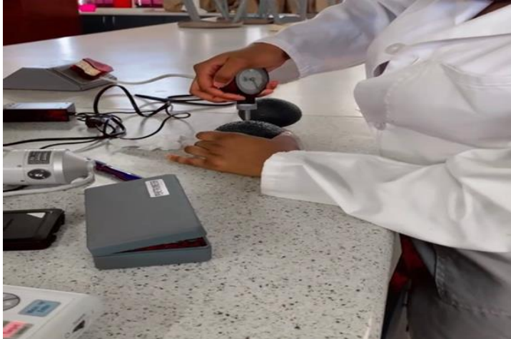
Figure 3.3 Firmness determination using penetrometer on ‘Hass’ avocado fruit
