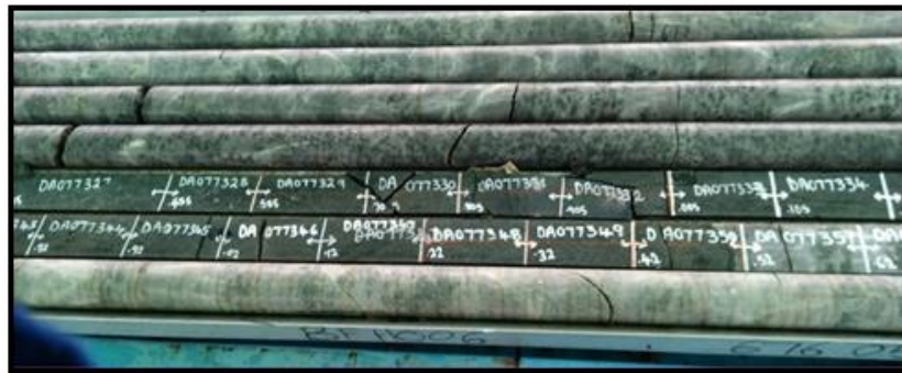
Figure 4.1: A photo of borehole BFH006D0 to show the half-core logged and sampled (not to scale).
