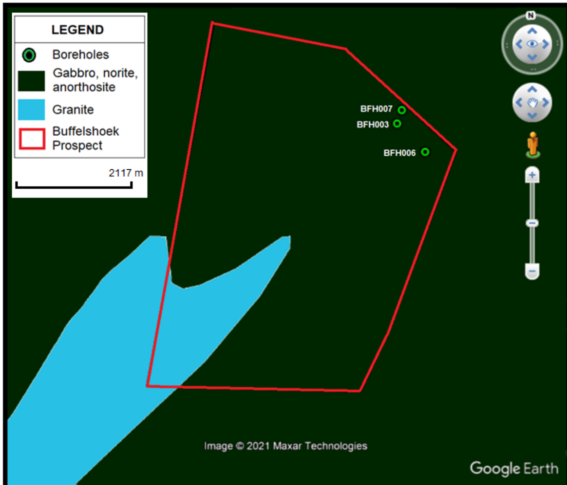
Figure 2.2: Local generalised geology of the Buffelshoek 368 KT (Buffelshoek) Farm showing the boundary of the farm and locations of the boreholes studied, geology from the Council for Geoscience (2021).
