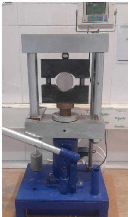
Figure 4.3 Brazilian tensile strength test.
