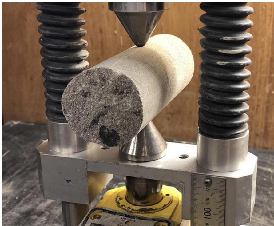
Figure 3.3 Point load test to determine point load strength.
