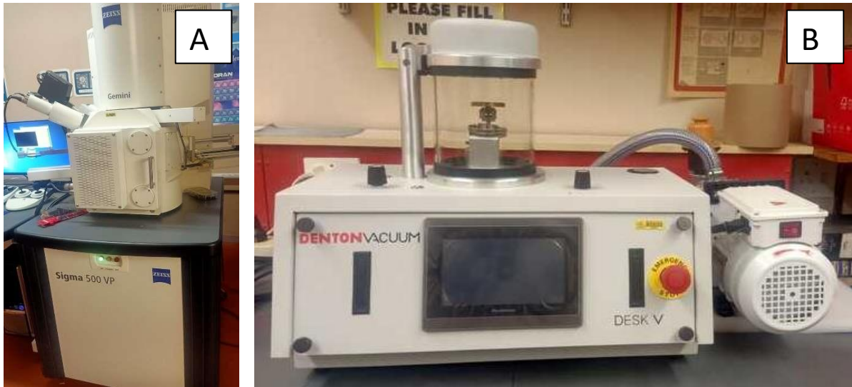
Figure 2.10: A = Zeiss Sigma 500VP scanning electron microscope, B = Quorum TM Q150T Emscope sputter coater.
