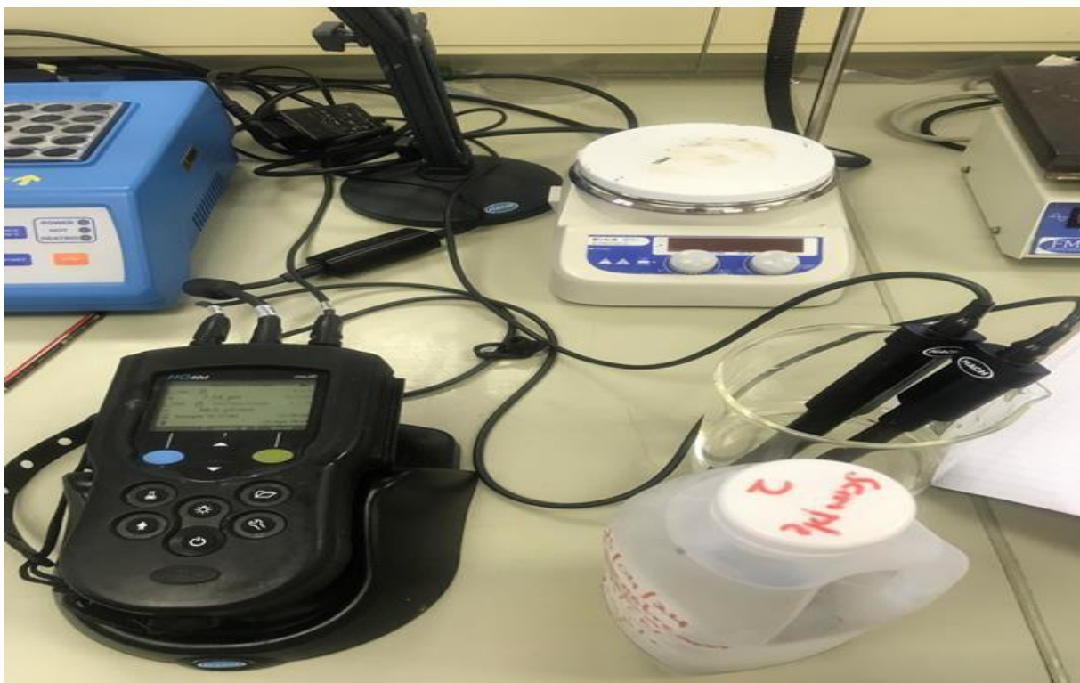
Figure 3.4: Analytical pH and EC assessment in water samples using a multi-parameter.
