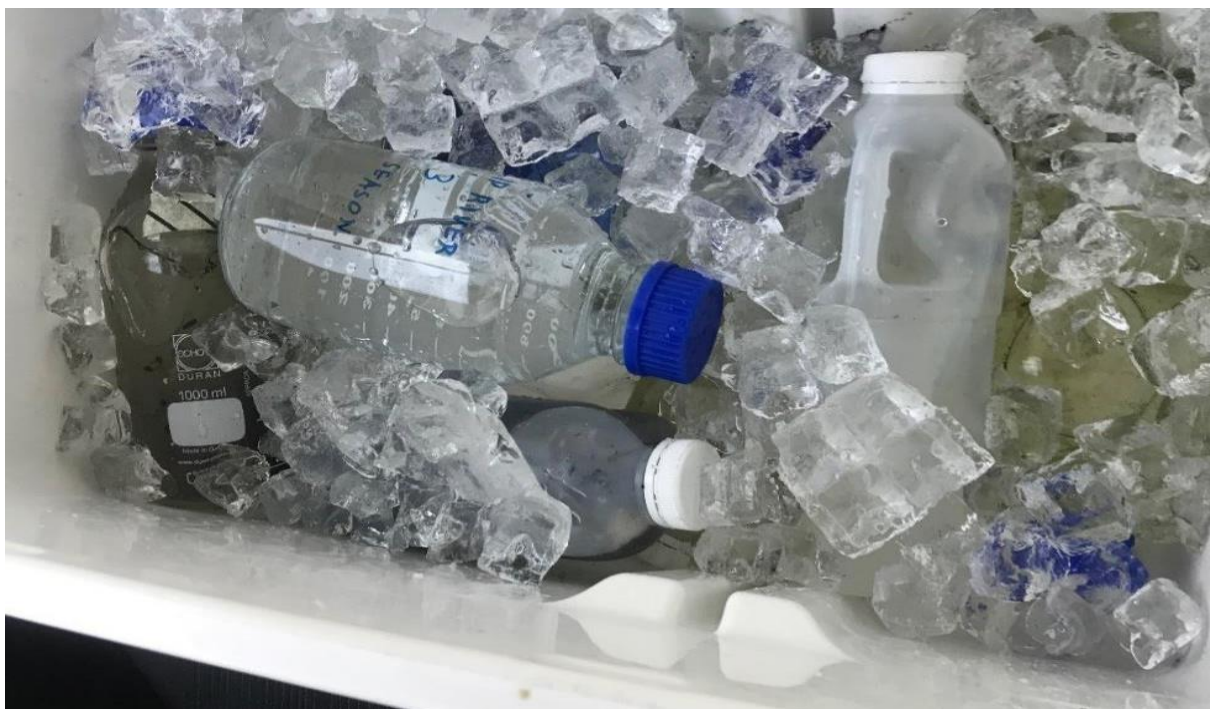
Figure 3.3: The preservation of water samples collected within the Klip River Wetland. Source: Mabale, 2024.
