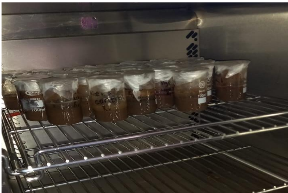
Figure 3.3: Samples ready for incubation at 37°C for 12 weeks bioremediation
