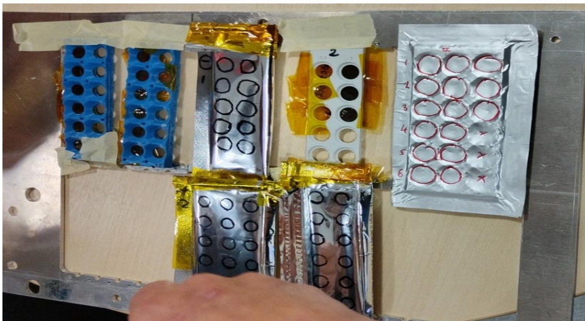
Figure 2-9. Different types of samples in a sealed foil on a rack ready for the beam.
