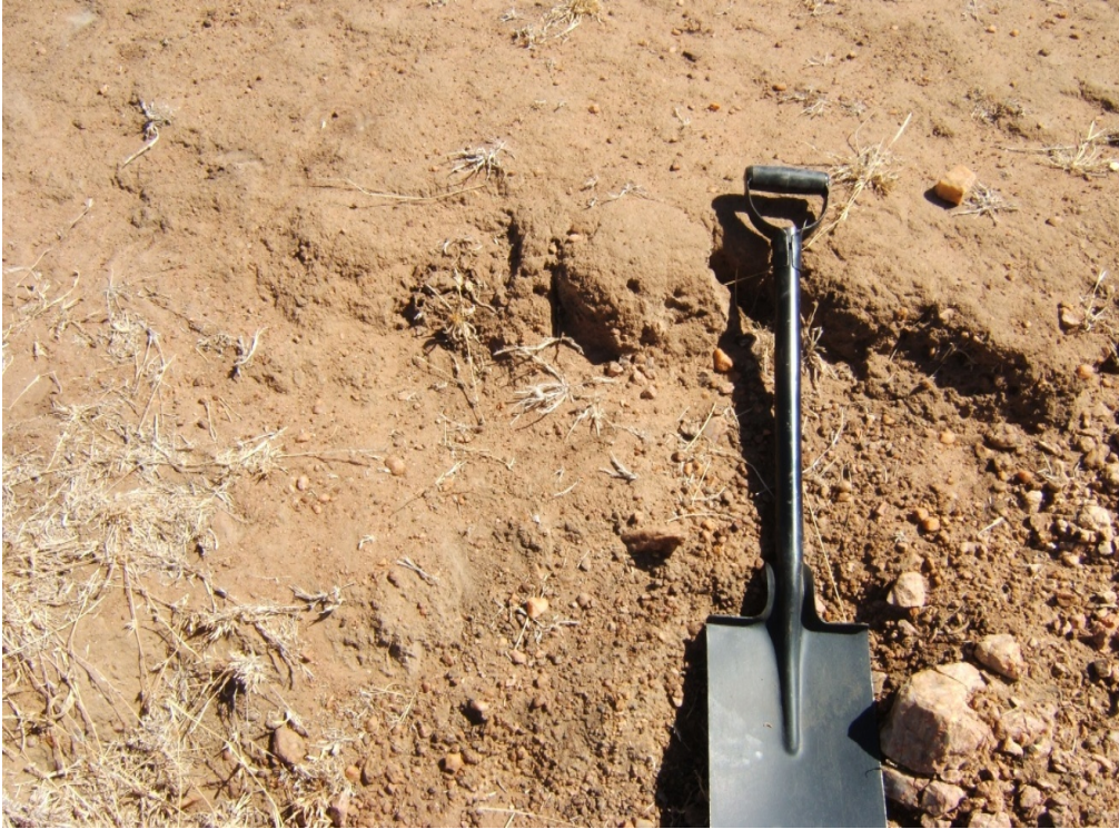
Figure 21: A photograph of soil type 3 showing a lithic horizon..
