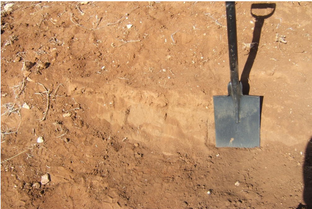
Figure 20: A photograph of soil type 3 ( Oxidic soil ) showing calcium carbonate nodules.
