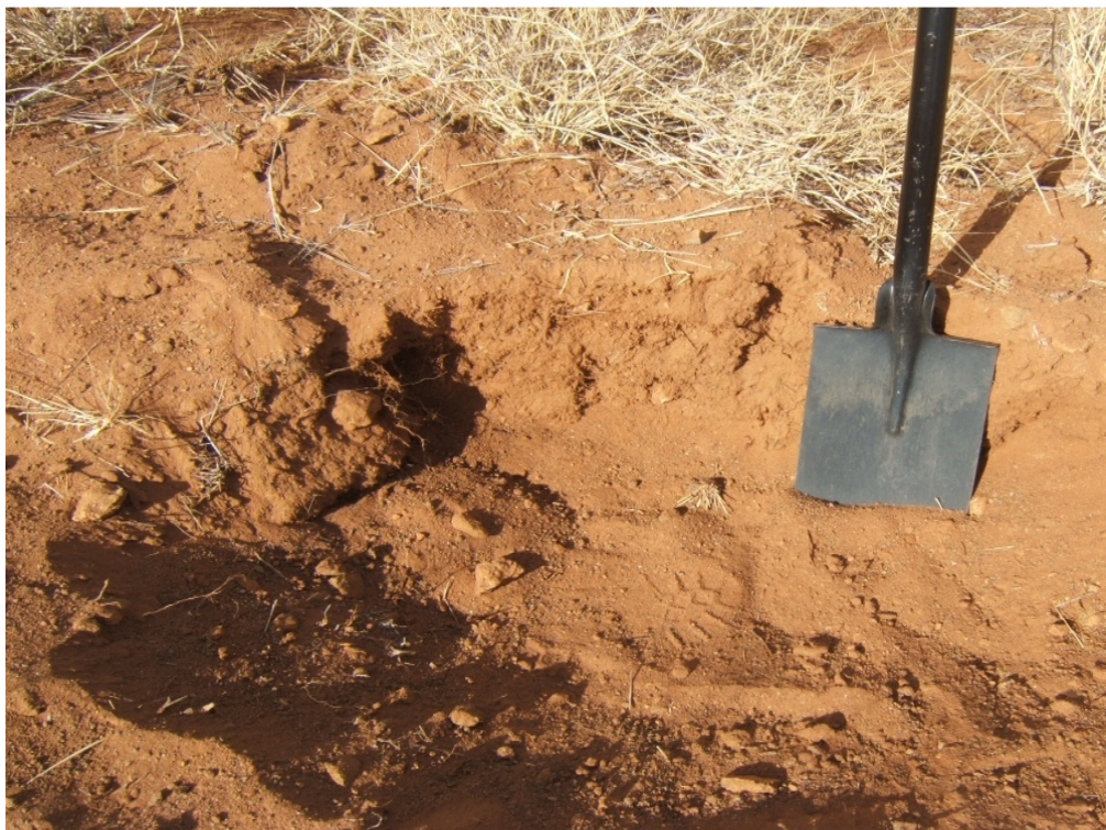
Figure 18: A photograph of soil type 2 showing a plinthic soil with less vegetation.
