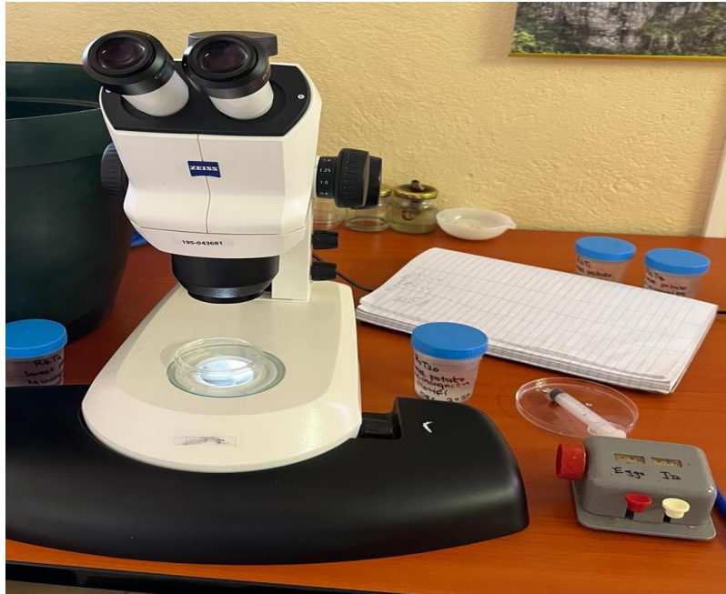
Figure 3.4 Eggs and second-stage juveniles (J2) counted out of 10 ml aliquot in a petri dish with the use of a stereomicroscope.
