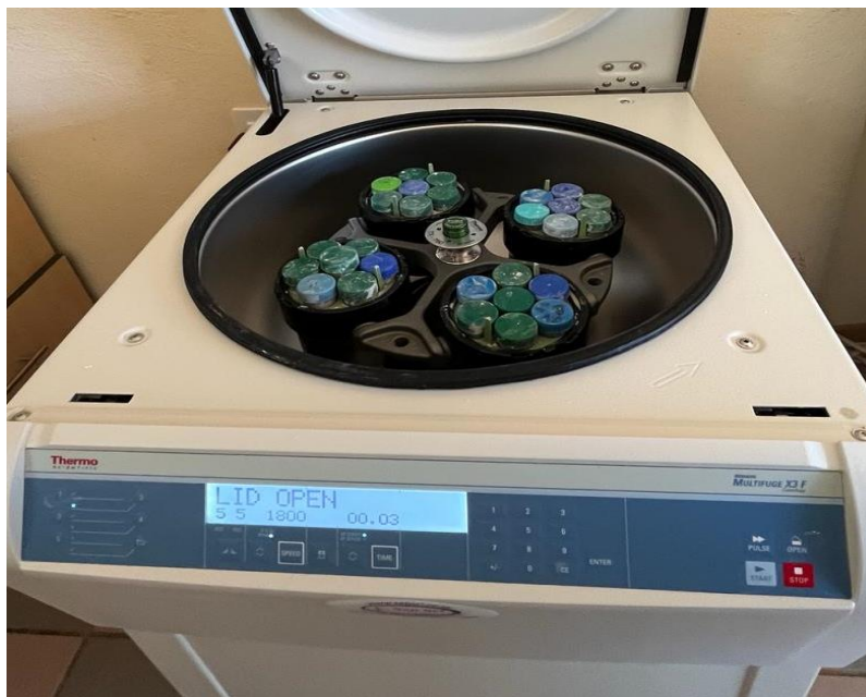
Figure 3.3 Nematode extraction using the sugar-floatation and centrifugation method.
